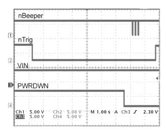
Figure 22. Boot Up Sequence of TTL Version (Vin= 5V) initiated by nTrig
